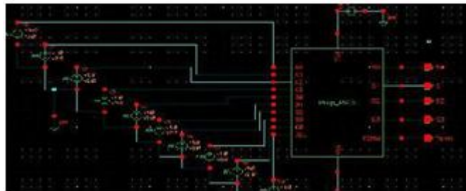
Figure 5 8-Bit Parallel Full Adder using SR-CPL
